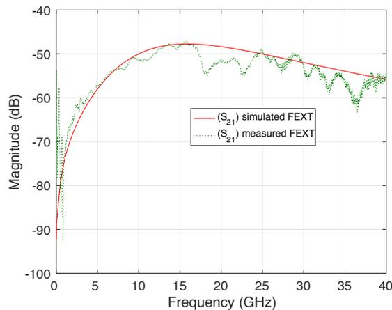
Figure 3: Measured and simulated crosstalk on two coupled modulators separated by a distance of  $115 \mu\text{m}$
