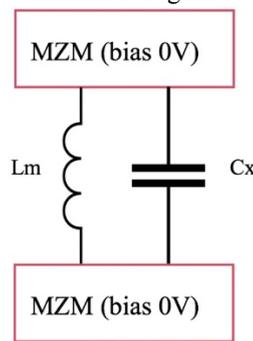
Figure 2: Schematic representation of the equivalent circuit model developed for the description of radiative crosstalk between MZMs
