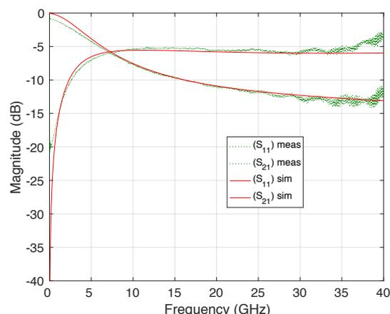
Figure 1: Comparison of the scattering parameters measured and simulated on a COBRA modulator
