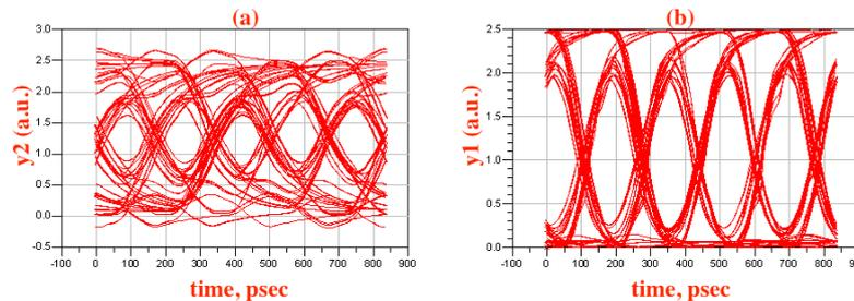
Figure 5: Comparison between electrical eye diagram (a) and electro-optical eye diagram (b) with crosstalk between MZMs up to -20 dB
