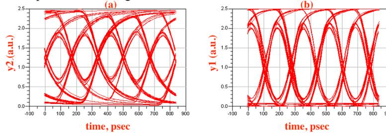
Figure 4: Comparison between electrical eye diagram (a) and electro-optical eye diagram (b) with crosstalk between MZMs up to -50 dB
