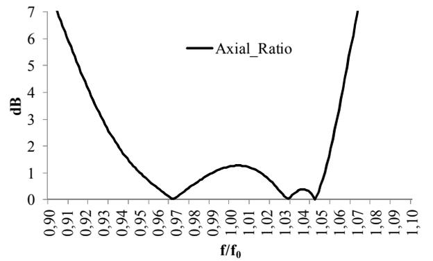
Figure 3. Axial ratio for the three layer polarizer in case of normal incidence ( $\theta = 0^\circ, \varphi = 45^\circ$ ).
