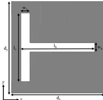
Figure 1. Geometry of the unit cell for each sheet of the multilayer circular polarizer:  $d_x$  and  $d_y$  are the periods along  $x$  and  $y$ , respectively,  $l_h$  and  $l_v$  are the horizontal and vertical slot lengths, respectively, and  $w_h$  and  $w_v$  are the horizontal and vertical slot widths, respectively.
