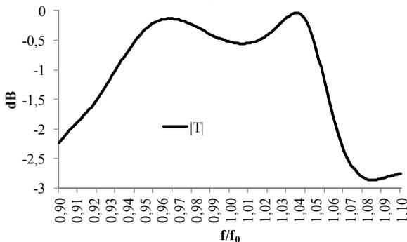
Figure 2. Power transmission coefficient for the three layer polarizer in case of normal incidence ( $\theta = 0^\circ, \varphi = 45^\circ$ ).
