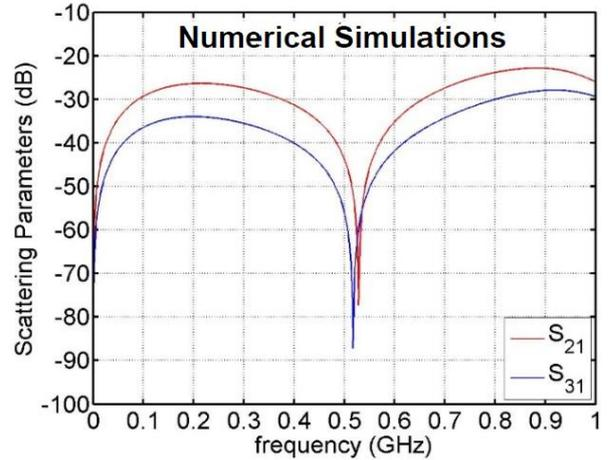
Figure 2: Transmission S-parameters versus frequency for adjacent striplines ( $S_{21}$ ) and for opposite striplines ( $S_{31}$ ).
